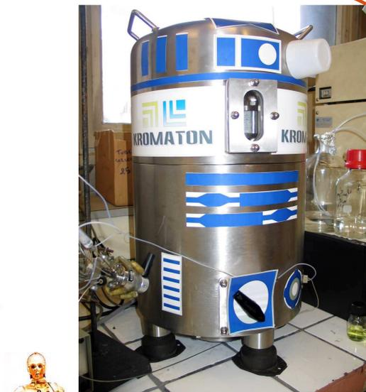
Two hydrostatic CCC columns: left, the Kromaton FCPC 250 that can hold different rotors including a 36 mL rotor; right, the Rousselet-Robatel-Decision-Design prototype (R2D2), a 32 mL hydrostatic column. The small inset picture gives the prototype scale.
